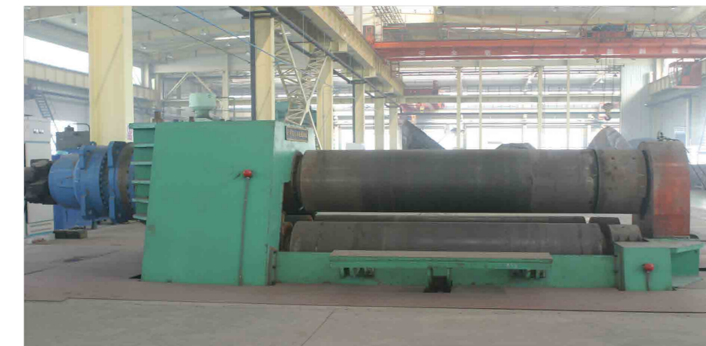
Rolling Machine (Max.rolling thickness 100mm)
