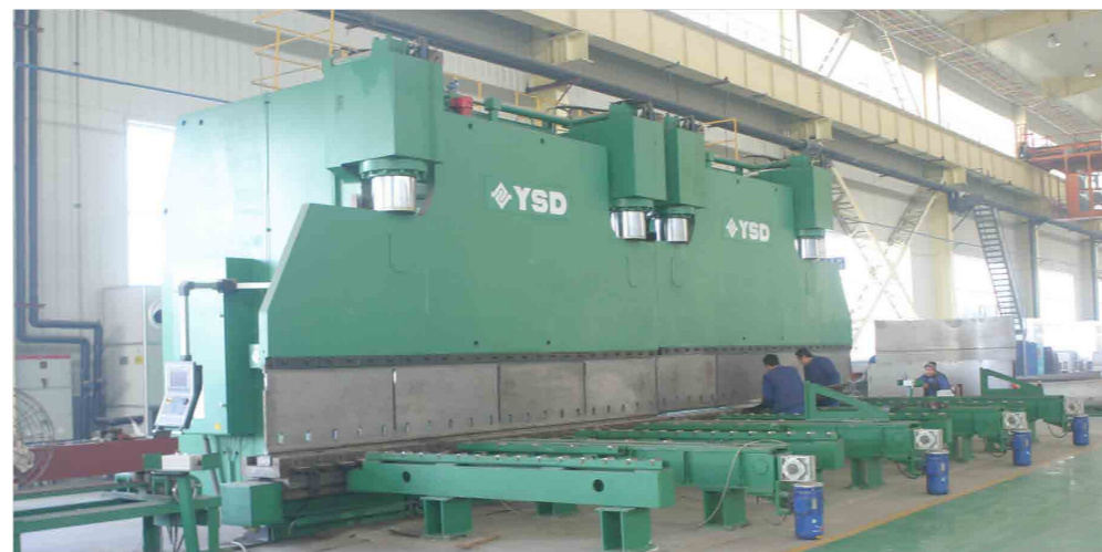
Dual Linkage Large Bending Machine (Max. processing length of 12m)
